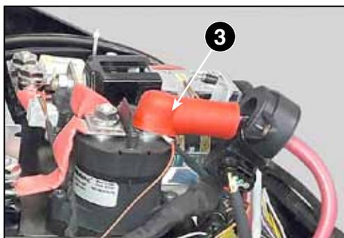
**⚠️ ⚠️ WARNING!** Always disconnect the red 48-volt battery cable (3) before starting any work that requires handling the cables and connectors.
