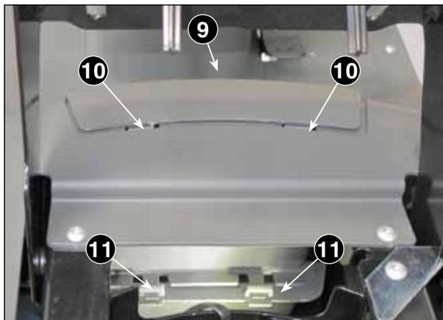
4. Remove the compartment (9), pushing it from the inside out.
