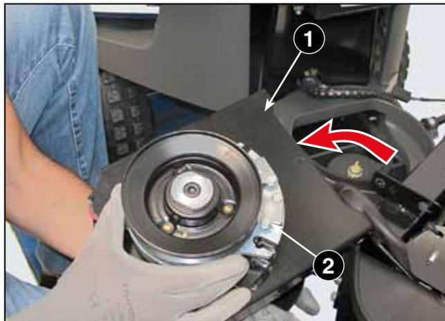
2. After removing the motor unit from the machine, turn the plate upside down (1) and place it on a suitable support to work comfortably on the pulley/clutch unit (2).
