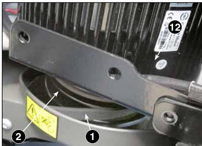
3. Turn the arm (3) of the tensioner towards the centre of the machine so that the belt (1) is free from the gallow pulley (4).
