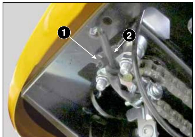
2. Carefully pull the cable out (2) until the connector comes out (3) of the frame hole and disconnect it.
