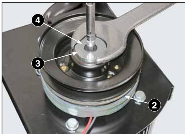
3. While holding the sleeve in place (3) with a 35 mm spanner, unscrew the central screw (4) and pull the sleeve (3) and clutch (2) out from the motor shaft..
