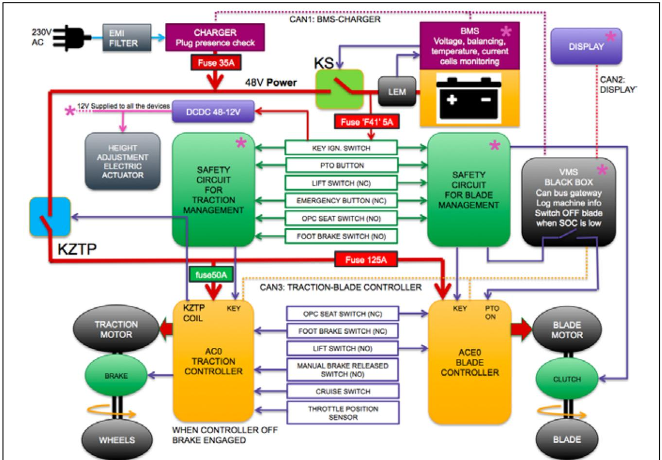
The block diagram shows the interaction of the main devices that make up the machine control system, the management of the power circuit, the CAN BUS communication system and electrical circuits that ensure total safety in the control of the electric motors.
