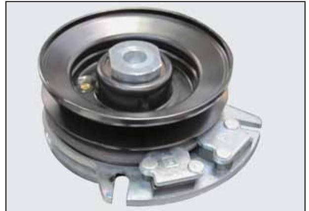
The clutch is engaged by applying current to the coil connection. This results in a current flowing through the coil, magnetizing the coil pulling the armature onto the rotor with sufficient force to hold the two pieces together, connecting the output and the input shafts firmly together. The force of the armature against the rotor pulls it away from the brake, hence releasing the brake.
