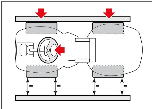
**NOTE** *With the wheels aligned and the steering wheel straight, the marking must be perfectly centred in the driving direction, in relation to the axis of the machine.*
