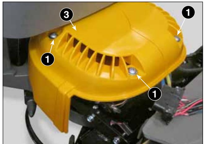
When mounting, complete in reverse the steps described above, making sure not to exceed the tightening of the screw (2) to avoid stripping the thread into the plastic of the of the left half shell
