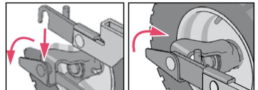
For safety purposes and to reduce the risk of physical injury in the event of accidental collisions and to protect important parts, the cutting deck is equipped with force limiters, such as:
