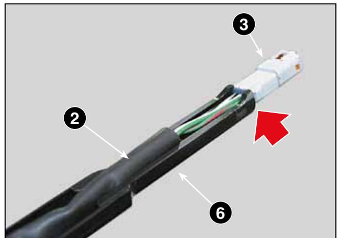
8. Make sure that the connector (3) remains in contact with the rod terminal, as shown in the drawing.
