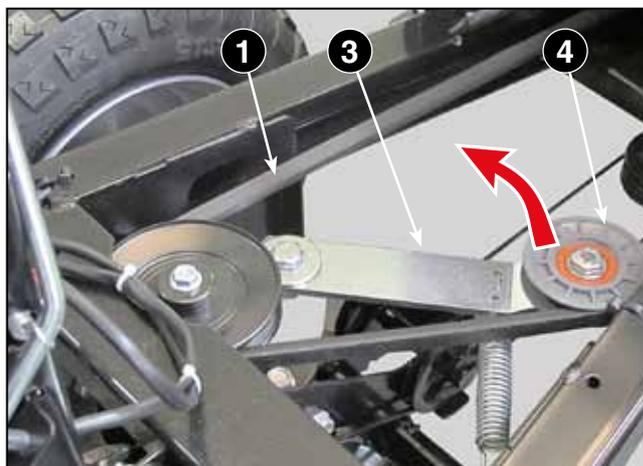
4. Once the belt (1) is completely loosened, it can be removed from the upper pulley (5) of the deflection axis.
