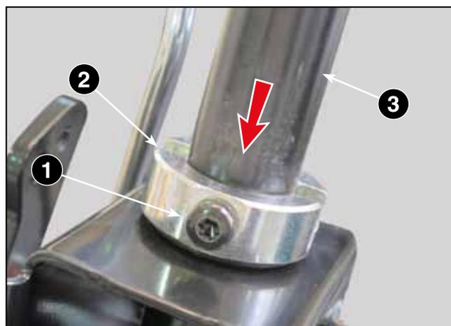
5. Remove the shaft from below (3).
