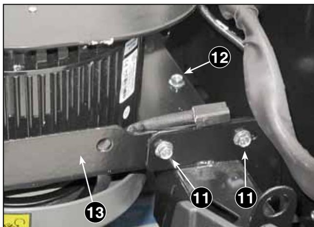
9. Slightly lift the front part of the plate (13) and, while holding it up, move it forwards so that the belt (6) is freed from the clutch pulley (14).
