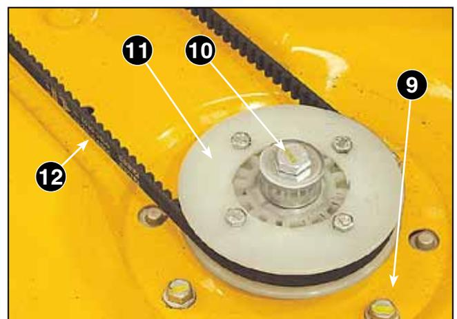
**NOTE** *The bearing housings cannot be removed and for individual spare parts are not available. If a malfunction is detected in the bearings, the entire bearing housing must be replaced.*
