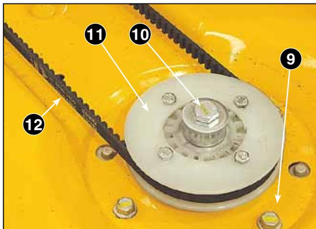
7. Reassemble the blade connection belt (12) and the pulley (11).
