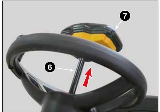
6. Push the display (7) slightly backwards, disconnect the connector (10) and then the display can be replaced, together with the cable (2) and the connectors (3) and (10).
