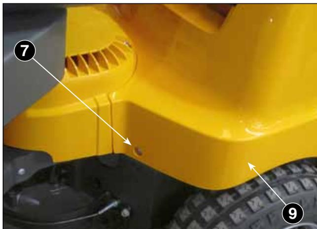
6. Unscrew the two rear screws (8) and remove the cover(9).
