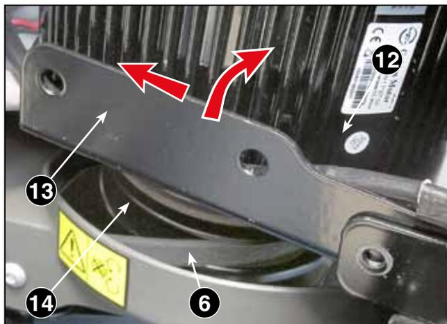
10. Carefully remove the plate (13) and the motor from the left side of the machine.
