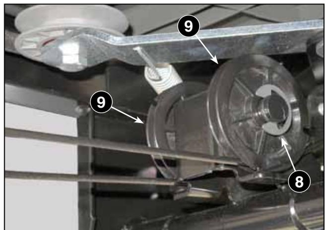
4. Remove the spring rings (8) and remove the two front pulleys (9).
