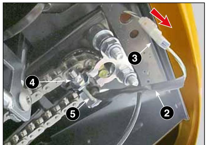
3. Undo the nut (4) and remove the screw (5) that axially stops the rod of the display .
