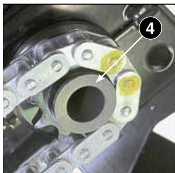
When reassembling the shaft (3) remember to reset the bush (4) at the shaft end, which is essential for the correct positioning of the display rod.
