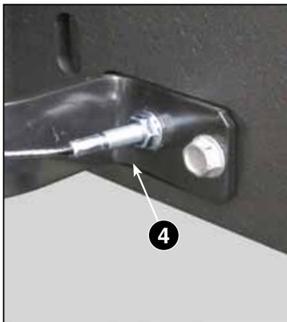
2. Unscrew both adjusters (4) on both the left and right sides of the machine.
