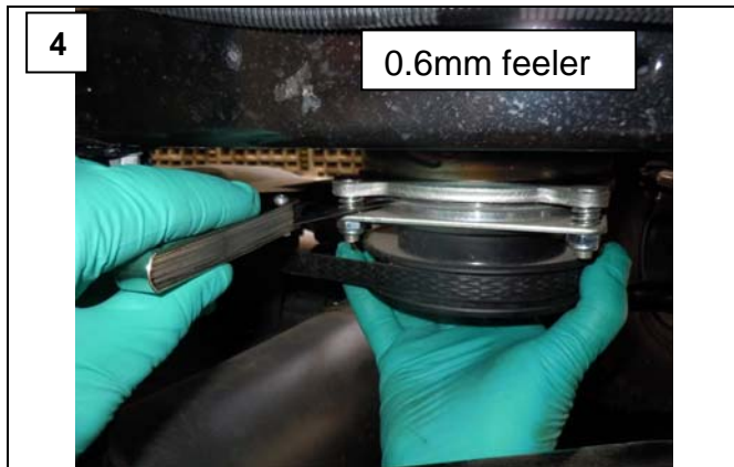
Rotate the clutch for a full 360° turn. 0.6 mm feeler shouldn't go in.
