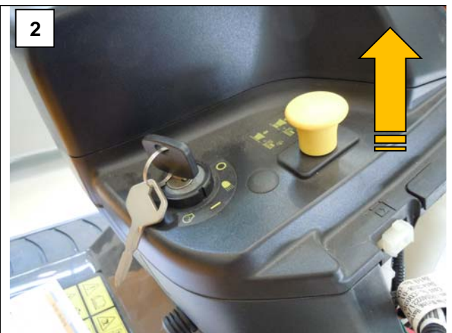
2 Turn the key to ON position and engage the blade, a click must be heard from the clutch
