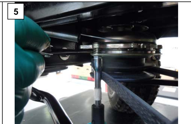
The air gap can be adjusted by tightening the 3 nuts. After adjusting please check the air gap according to step 3 and 4.
