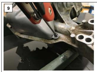
Secure the expansion tank by tightening the selftapping bolt.
