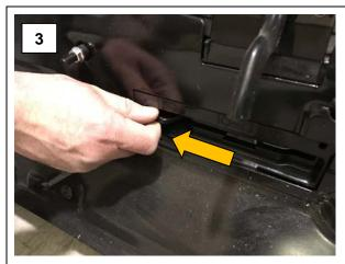
Close the by-pass valve by setting the lever on the closed position
