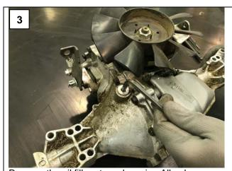
Remove the oil fill port cap by using Allen key.
