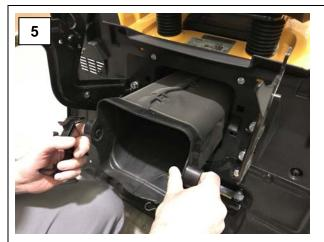
Stop the engine, remove the discharge chute to have access to the transmission area
