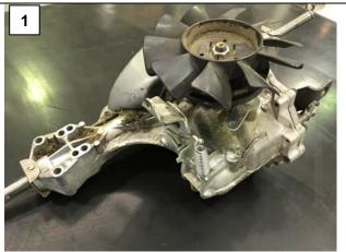
Remove the transmission from the vehicle – refer to the workshop manual (chapter 5.6a) for step-by-step instructions.
