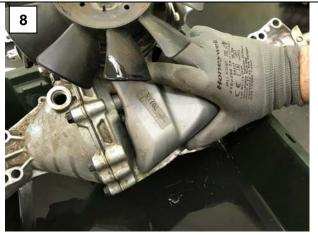
Push the tank opening over the O-ring to ensure a proper seal and put the vent hose in his position.
