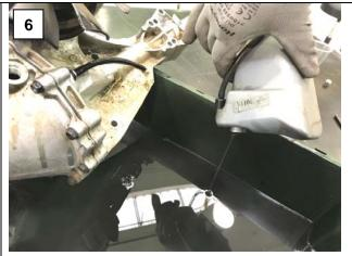
Remove the tank and drain out the oil from the tank. Do not remove the vent cap from the tank. Do not remove the tank hose or O-ring unless replacement is needed.
