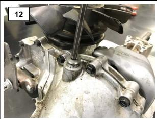
Install the oil fill port cap making sure the O-ring is correctly inserted in the cap thread and assemble the transmission to the vehicle.
