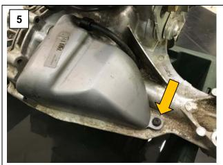
After the oil is drained from the transmission remove the expansion tank by removing the self-tapping bolt (Torx T25 key needed)
