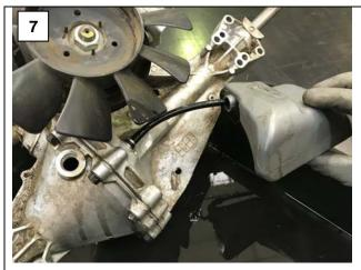
Install the tank by first inserting the hose into the opening in the expansion tank.
