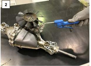
Clean the expansion tank and oil fill port areas of any debris by mean of a flow of compressed air or by using a brush.
