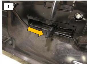
Open the by-pass valve by setting the lever on the open position.
