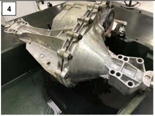
Position the transmission so that the oil will drain completely out of the housing.
