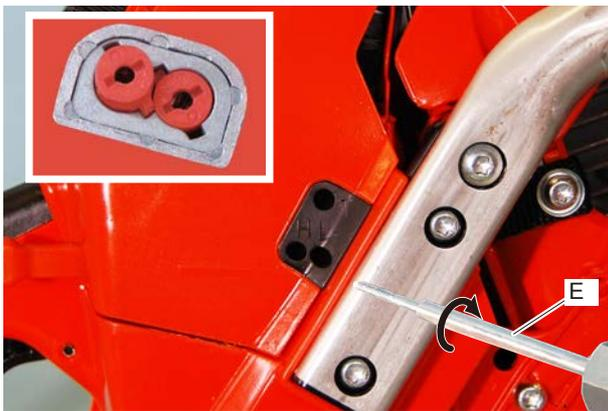
3. Remove the tool from limiter cap by turning clockwise, leaving the limiter cap in place.
