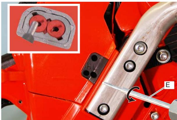
2. Screw limiter cap tool (E) counterclockwise into center hole of limiter cap until tab of limiter cap comes out of locating slot as shown in left below picture.
