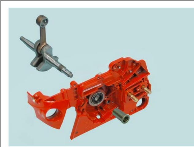
1. Apply grease on the oil seal lip and heat up the main bearing using a heat gun.
