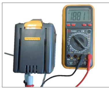
If the measured value is out of the range given it means that the battery is damaged.
